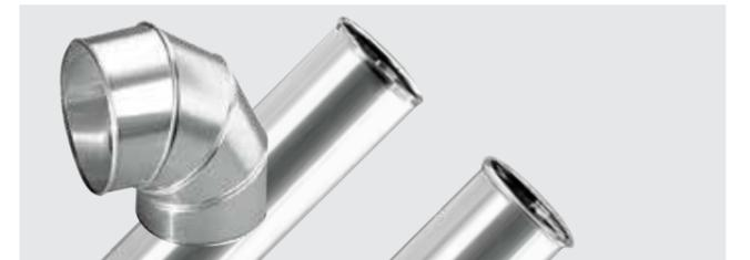
99.5% PURE ALUMINIUM SHELL and 90° ELBOWS with a thickness ranging from 0,6 and 0,8. MT 500: male and female ball swaged edges calendered tube, with reinforced length-wise drilled sealing system. Length: 1000mm. CU 501: 90° preformed segmented elbows with female-female ball swaged edges.
